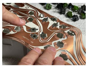
3. Work your way to the left, insert the two that are almost in a vertical row and then the last one that is directly above the vertical electrical connector until they are all in the same places that they were before you removed them.
