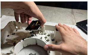
With all these components removed, can you see the instrument cluster light bulbs & sockets along with the metal clips that the threaded studs on the back side of the gauges slide into to make their electrical connection. Before proceeding, make sure you have a photo of the backside of the cluster showing where the metal clips light bulb/sockets are installed.
