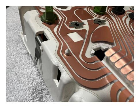
Wait to press the PCB into place over the right side locator peg until after you have made the final connections when installing the cluster back into the car.
