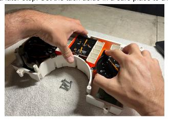
5. Repeat the same process as you did for the tachometer for the speedometer and set it aside in a safe place to avoid damage.
