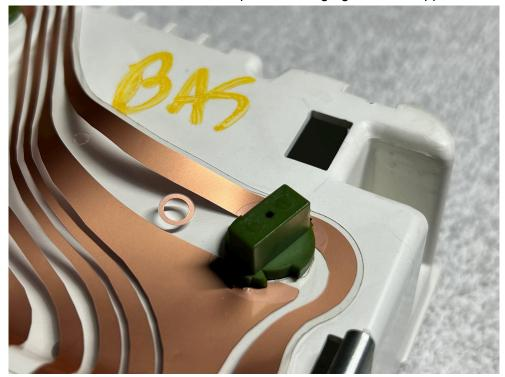
2. Go back and forth from left to right, top to bottom. As you get to the outermost sockets, you may have to gently apply pressure one direction to get the hole in the PCB to line up with the hole in the instrument cluster housing.
